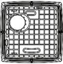
3. Hold the mounting bracket against the ceiling (or wall) so the arrow located on the mounting plate is pointing to the left. (The circular shape will now be in upper right-hand corner). Trace around the insides of the mounting slots.
