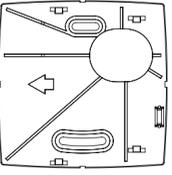
5. Using a 3/16" (5 mm) drill bit, drill a hole through the center of the oval outlines you traced in step #3.
