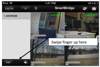
Swipe finger as shown in the picture above to obtain PTZ controls in Landscape view. Swipe finger in the same position in a downward motion to hide the PTZ controls.
